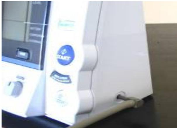
For all cuff sizes small, medium, large, and thigh connect the air tube to the main unit by attaching the air plug to the base of the air connector. Connect the cuff to the air tube attached to OMRON unit Wrap and secure the appropriate cuff to the participant's upper right arm as set out in section 12.2.7, above.
