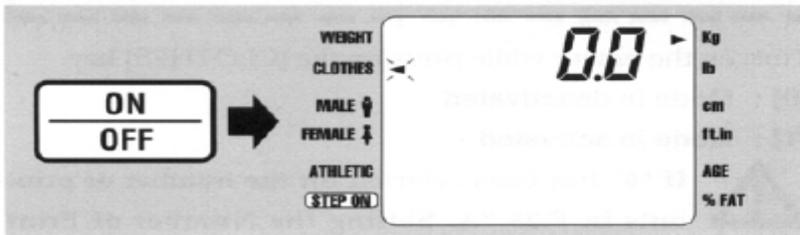
Press ON/OFF key to turn the machine on. Wait until 0.0 and an arrow appear on the screen. Check that the arrow points to “Kg”. If arrow point to “lb”, press the Kg/Lb key on the control panel and the arrow will shift to “Kg”
