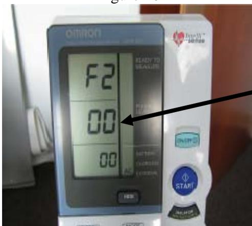
If needed push the DEFLATION (deflation control)/Measurement Result Display Switch Button and change the set value to 0 sec waiting time. Push the START button and F3 function is displayed in the first window and inflation interval 30 second time is displayed in the bottom window (Figure 11).
