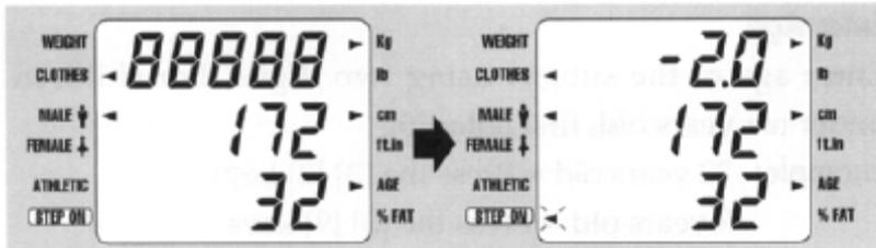
Mistakes may be corrected by pressing the [CE] key. Pressing this key repeatedly will allow correcting the previous information
