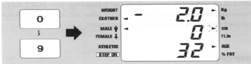
Enter age of participant using the numeric pad of the control panel. After age is entered, the arrow will direct you automatically to enter the height.
