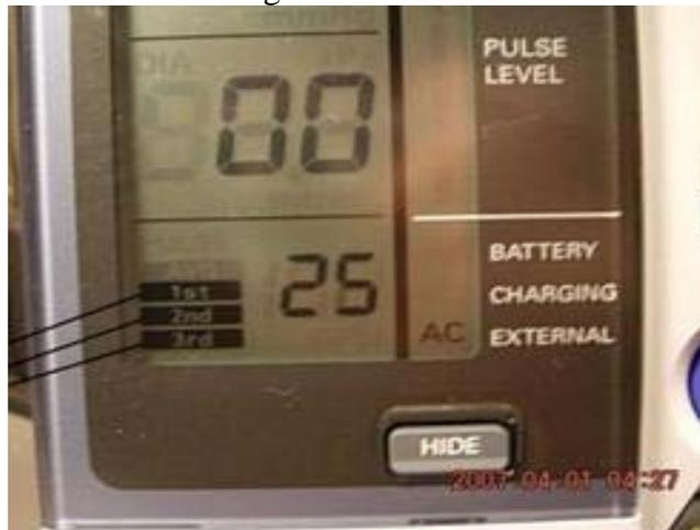
After each inflation and deflation the systolic blood pressure, diastolic blood pressure and pulse rate will be displayed in the top, middle and bottom sections of the LCD screen.
