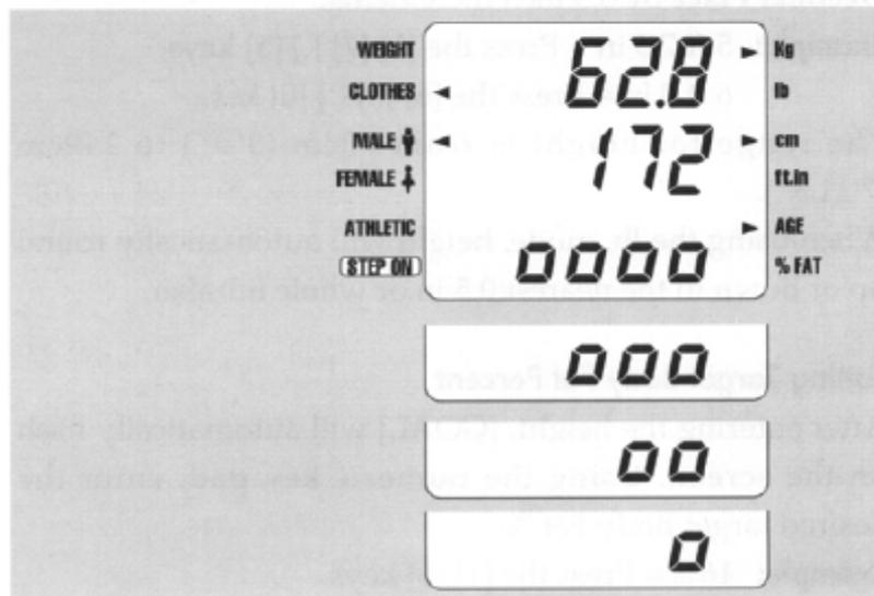
Weight will be displayed on the upper section of the screen. After weight stabilizes, impedance measurement is taken. Bubbles “oooo” will appear on the bottom half of the screen as these measurements are being analyzed. Once body composition measurements are ready, the bubbles will disappear one by one. Record weight and each body composition measurement including impedance on the Anthropometry form. Ask the participant to step off the scale.
